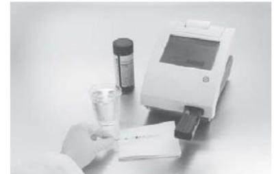
8. When the urine results are ready, the Results screen is displayed. The first page of the test results are displayed on the screen and the test table and strip are automatically pushed out of the analyzer.
